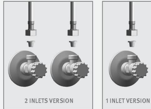
**MAKE SURE THAT THE FILTER(S) IS/ARE INSTALLED BETWEEN THE FLEXIBLE PIPE AND THE SHUT OFF VALVE (ANGLE VALVE) (NOT SUPPLIED).**
